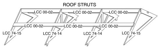
Diagram above shows the roof truss structure as it was assembled outside of the engine shed. We recommend not to assemble it outside of the shell unless a removable roof is required.
