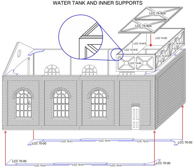
After the shell have been assembled and all of the decoration pieces shown on previous page have been glued to the shell assemble the water tank and glue it to the back end of the shed. Water tank should be glued to the engine shed in such a way that the protruding decoration elements are even on all three sides.
