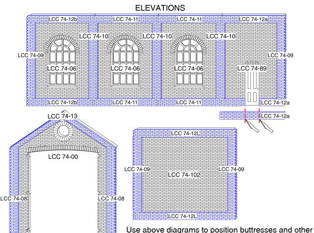
to first assemble the shell of the building composed of LCC 74-00, LCC 74-102, and LCC 74-06 etc. Substitute LCC 74-18 on one of the sides for LCC 74-89. Elements on the right and left edges of wall and gate panels should be protruding about quarter of a brick outside of the panel. Note that a space needs to be cut in one of LCC 74-12a elements for the door. This can be done
