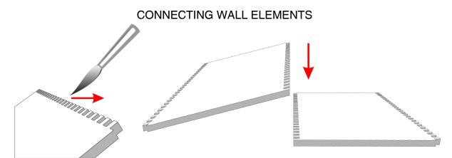
Recommended way of gluing parts together is to apply PVA glue to the interlocking bricks working from back of the part to the front. This ensures there will be no glue overflow on the front, visible side.
