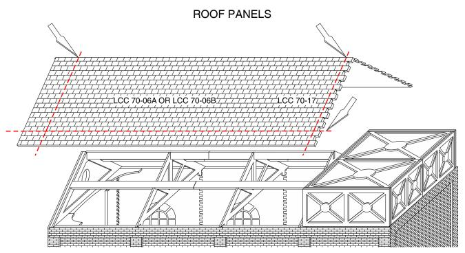
Glue LCC 70-17 to each LCC 70-06A and LCC 70-06B to form the roof tiles panel blanks. Leave to dry.
